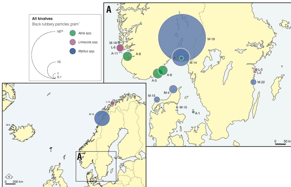
**Figure 43: Combined results for the species containing black rubbery fragments from the Nordic environment; *Abra nitida* (A), *Limecola balthica* (L) and *Mytilus* spp. (M). Asterisk \* refers to upper quantification limit for particles at site M-19.**
