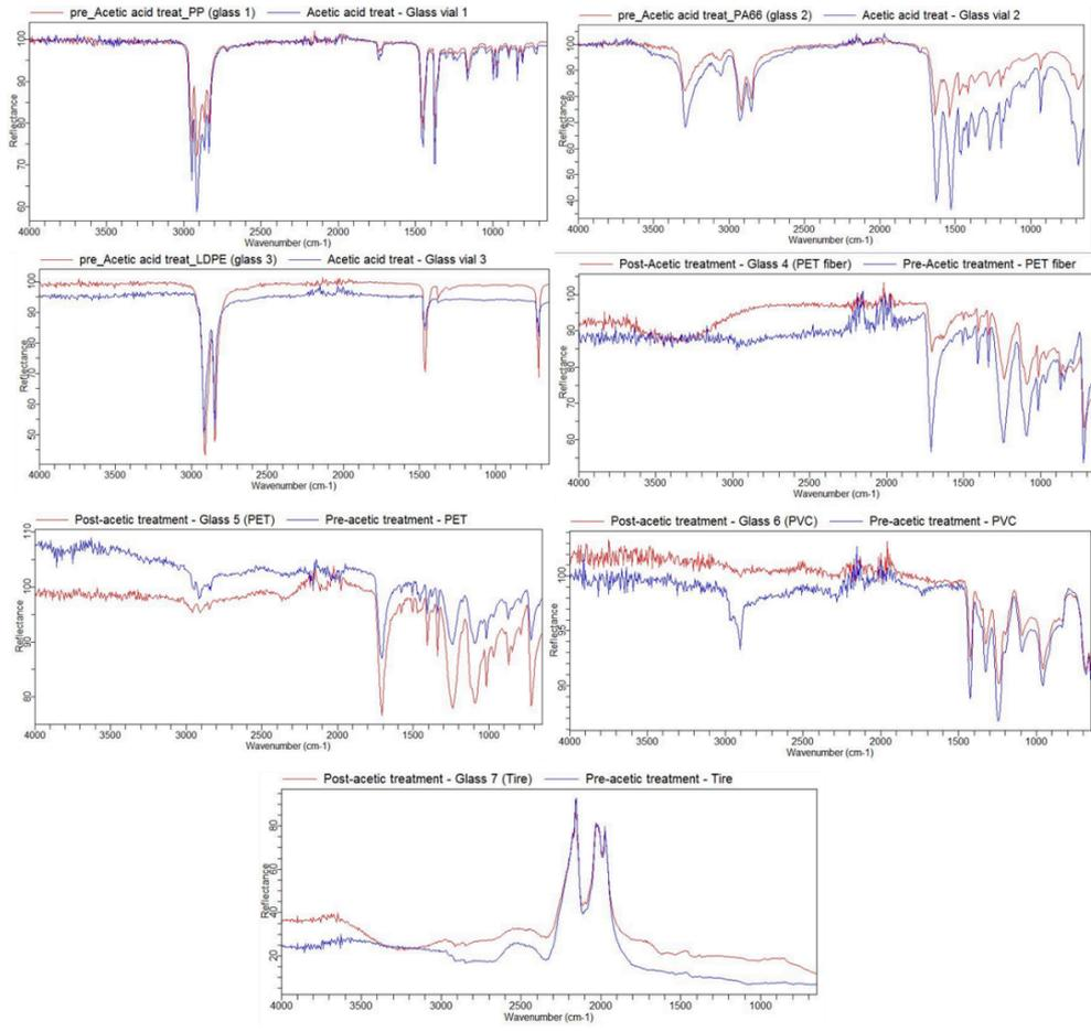
**Figure 44: FT-IR spectra of the seven polymers tested for impact from KOH + acetic acid. See Table 18 for more information.**
