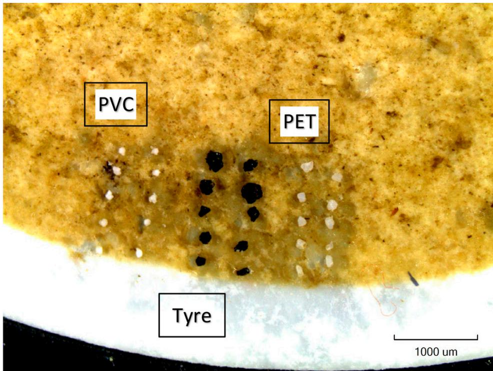
Figure 16: Illustration from recovery test with *Mytilus* spp. tissue present. Ten particles of PVC fragments, tyre particles and PET fragments. One PET fibre is also present in the lower right corner.
