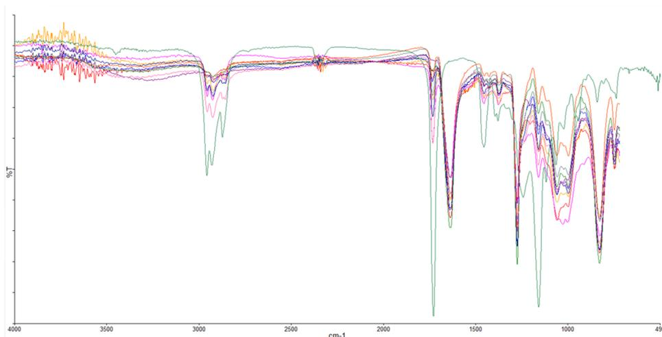
Figure 48: FT-IR Spectrum where green is the reference spectrum of polyacrylate and the rest are spectra for suspected polyacrylate in the samples.
