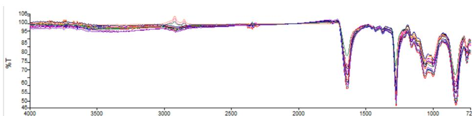
Figure 47: FT-IR Spectrum from all 15 spectra obtained from the blank.
